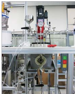
View Cell Reactor
