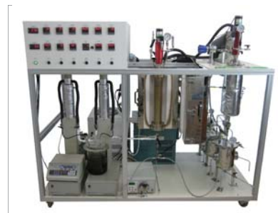
Supercritical Methanol Trans Esterification
