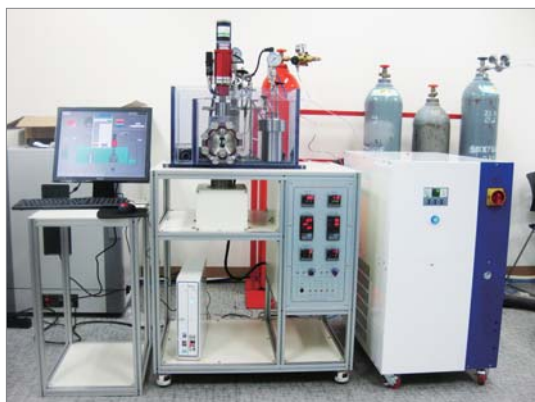
Hydrate Reactor System
