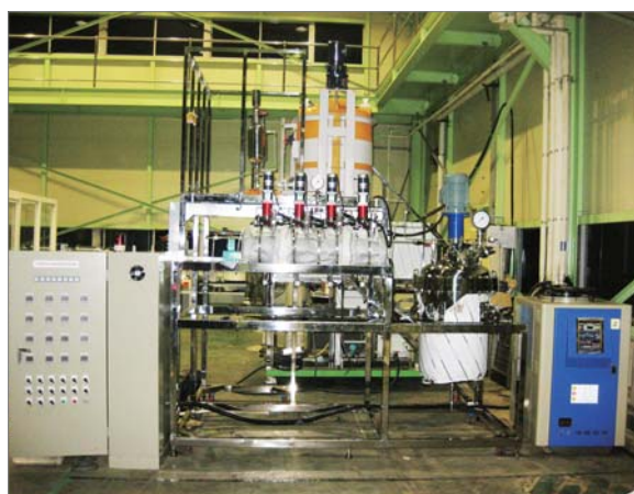
Continuous Leaching Reactor System
