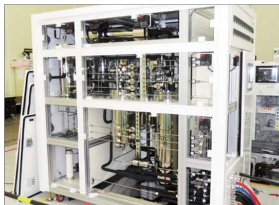
CO 2 Recovery System
