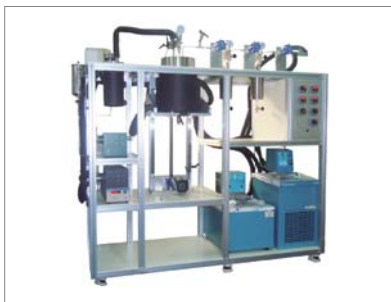
Supercritical Extraction System
