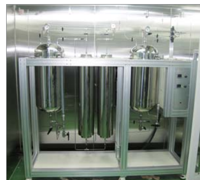
Liquid Purification Column
