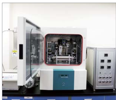
Core Cell System with Oven
