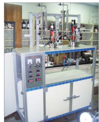
EO Gas Reactor System
